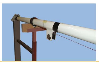
Fix in place at the butt to allow it to rest on the collar as it holds by the mast step and deck of the boat. Mark the point A.
